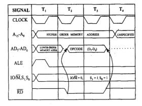
Figure 1.2 Timing Diagram for Opcode Fetch Machine Cycle
