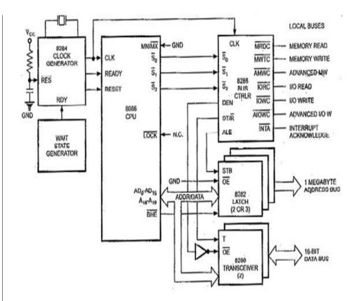
Figure 2.4 Maximum mode functions of 8086
