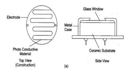
Figure 14.3Schematic structure of the photoconductive cell
