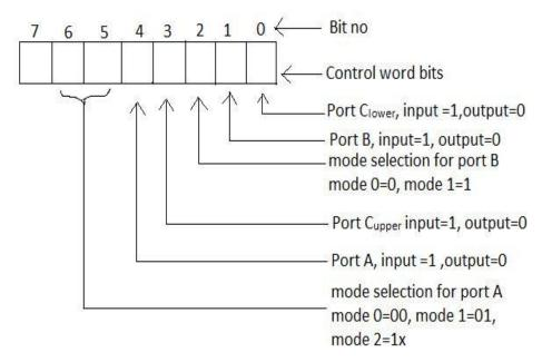
Figure 8.1 Control word bits for Intel 8255
