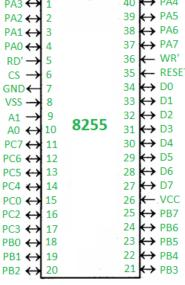
Figure 8.3Pin configuration of 8255
