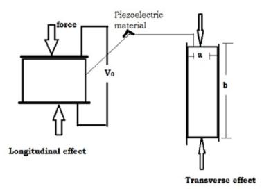
Figure 14.4 Block diagram of crystal in a transducer
