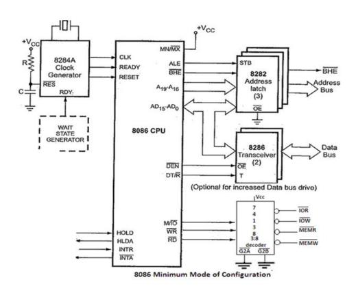
Figure 2.5Minimum mode functions of 8086
