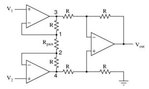
Figure 11.1Block diagram of Instrumentation amplifiers
