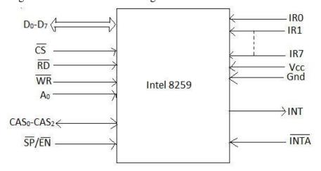
Figure 8.4 Schematic diagram of Intel 8259
