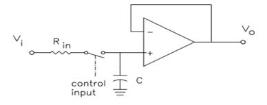
Figure 11.2Basic circuit of sample and hold circuit
