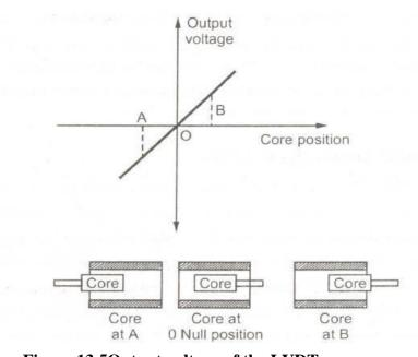
Figure 13.5Output voltage of the LVDT
