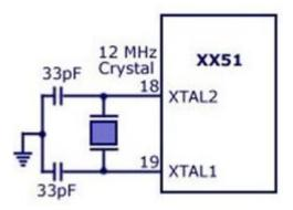
Figure 5.5 8051 clock circuit
