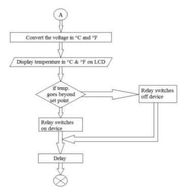
Figure 10.3Flow chart for the microprocessor based temperature monitoring and controlling
