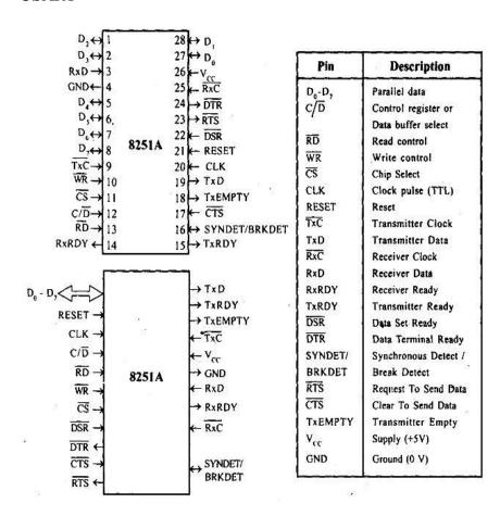
Figure 9.3 Pin description of Intel 8251 USART
