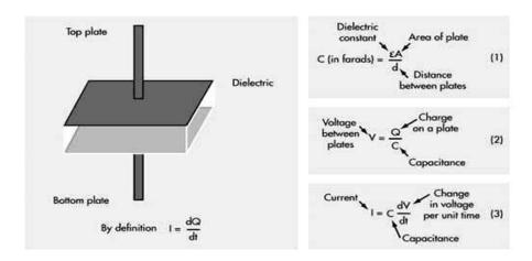
Figure 13.3 Parallel plate capacitor
