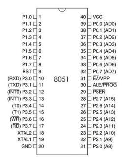
Figure 5.2Pin diagram of 8051 microcontroller
