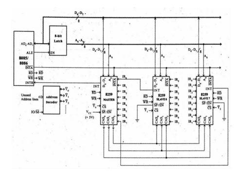
Figure 8.6 Scheme for interfacing 8259 with 8085
