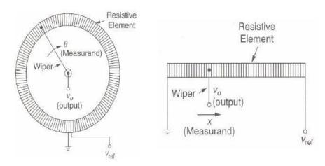
Figure 13.2 Types of potentiometer
