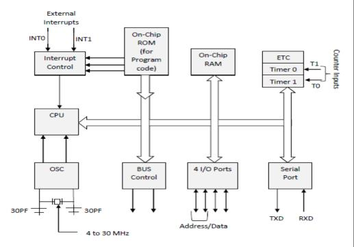
Figure 5.1 Block Diagram of 8051 Microcontroller
