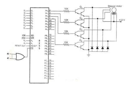
Figure 10.4Interfacing stepper motor with 8085
