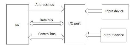
Figure 7.7 Interfacing of I/O device through I/O port
