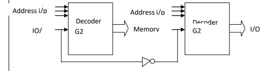
Figure 7.3 Scheme for I/O interface
