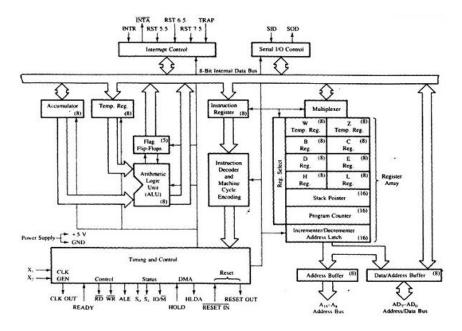
Figure 1.1 Architecture of Intel 8085
