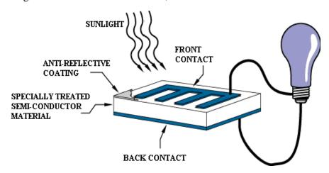
Figure 14.2 Block diagram of photo-voltaic cell
