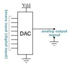
Figure 11.4 Block diagram of Digital to Analog Converter
