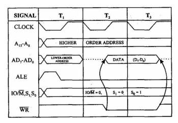
Figure 1.4 Timing Diagram for Memory Write cycle
