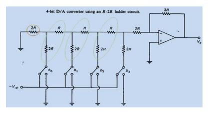
The above figure shows the 4-bit R-2R ladder DAC. In order to achieve high-level accuracy, we have chosen the resistor values as R and 2R. Let the binary value B3 B2 B1 B0, if b3=1, b2=b1=b0=0, then the circuit is shown in the figure below it is a simplified form of the above DAC circuit. The output voltage is V0=3R(i3/2)=Vref/2
