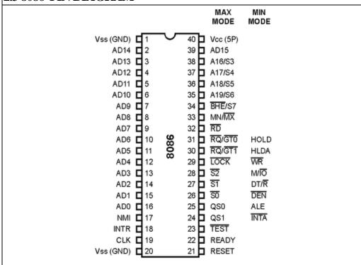
Figure 2.2 Pin diagram of 8086
