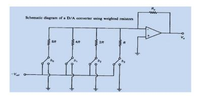
In the voltage domain, that is if the input signals are voltages, the addition of the binary bits can be achieved using the inverting summing amplifier shown in the above figure.
