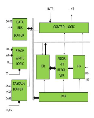
Figure 8.5 Internal architecture of 8259
