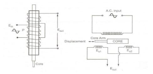
Figure 13.4 Skeletal picture of the LVDT
