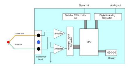
Figure 10.2Scheme for temperature monitoring and controlling
