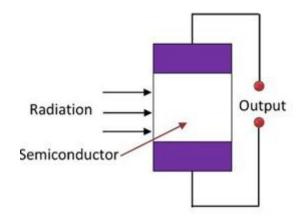
Figure 14.1 Block diagram of photoelectric transducer
