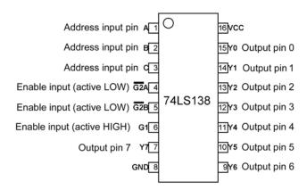
Figure 7.1 Pin diagram of 74LS138
