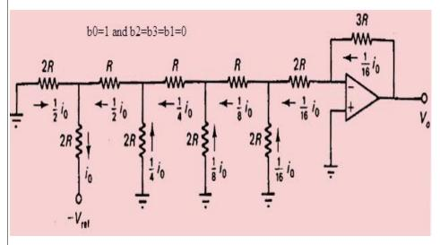
In this way, we can find that when the input data is b3b2b1b0 (where individual bits are either 0 or 1), then the output voltage is
