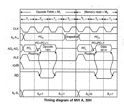
Figure 1.3 Timing Diagram for Memory Read
